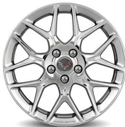
RPO R86 19" x 8.5" front and 20" x 10" rear Motorsports polished-aluminum
