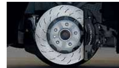
Black calipers standard on Grand Sport and available on Stingray and Z06 7 (Brembo ® slotted brakes included with available Z51 Performance Package shown)
