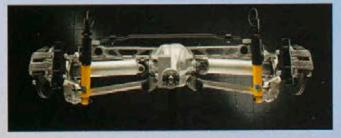
FULLY INDEPENDENT REAR SUSPENSION A unique 5-link independent rear suspension with a transverse monoleaf spring helps put power to the pavement.
