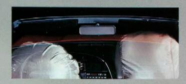
STANDARD DUAL AIR BAGS The driver- and passenger-side air bags supplement the protection of safety belts in certain moderate to severe frontal collisions. Remember to always wear safety belts, even in cars equipped with air bags.
