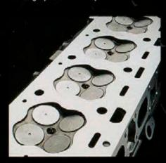
32 VALVES, 405 HP The all-aluminum LT5 V8 features four overhead camshafts and four valves per cylinder for excellent volumetric efficiency through a wide rpm range.
