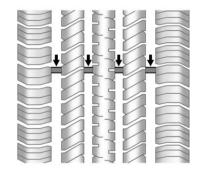
Treadwear indicators are one way to tell when it is time for new tires. Treadwear indicators appear when the tires have only 1.6 mm (1/16 in) or less of tread remaining. See *Tire Inspection on page 10-65* and *Tire Rotation on page 10-66*.
