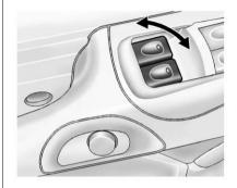
The power window switches are located on each door.
