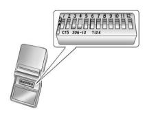
To verify that the garage door opener is a Fixed Code unit, remove the battery cover on the hand-held transmitter supplied by the manufacturer of the garage door opener motor. If there is a row of dip switches similar to the graphic above, the garage door opener is a Fixed Code unit. If you do not see a row of dip switches, return to the previous section, "Programming Universal Home Remote – Rolling Code."
