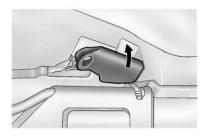
To unlock the release latches on the front of the roof panel, grasp each handle and pull it outward.
