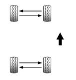
Use this rotation pattern if the vehicle has different size tires on the front and rear and they are non-directional.
