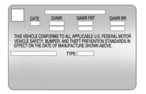
A vehicle-specific Certification label is attached to the rear edge of the driver door. It tells you the gross weight capacity of your vehicle, called the Gross Vehicle Weight Rating (GVWR). The GVWR includes the weight of the vehicle, all occupants, fuel and cargo. Never exceed the
