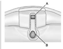
To unlock the rear of the roof panel's rear release latch, press the back of the release handle (B). Then press the button on the front of the release handle (A).
