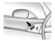
On vehicles with the memory feature, the controls on the driver door are used to program and recall memory settings for the driver seat, outside mirrors, and the telescopic steering column, if equipped.
