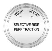
This knob is on the center console. Turn it to select the suspension of vour choice. The knob will return to the center position when released. The switch will illuminate the current suspension setting.
