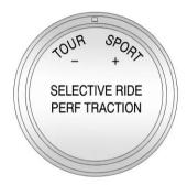
To select a mode while in Performance Traction Management, turn the knob on the center console.
