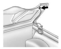
Tilt the driver seat forward and press the tonneau cover release button. After pressing the release button, the driver and passenger door glass will retract to the full-down position. If battery power has been lost, see Step 7 under "Lowering the Manual Convertible Top" in this section.
