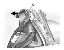
Pull the convertible top up by firmly gripping the front edge (A) near the center and applying a brisk upward and forward motion to get the top in the full-up position.
