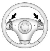
The Manual Paddle Shift system can be used in D (Drive) or S (Sport Mode). The system is activated by pushing the paddle, above the steering wheel spokes, to manually up-shift to the next gear, or pulling on the paddle, behind the steering wheel spokes to manually down-shift. The current gear will be displayed in the Driver Information
