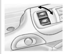
Pull up or press down on the front of the switch to raise or lower the window. Retained Accessory Power (RAP) allows you to use the power windows when the ignition is off. For more information, see Retained Accessory Power (RAP) on page 9-21.
