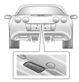
Press the hatch/trunk release touch pad with the keyless entry transmitter within range.
