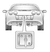
From outside the vehicle, use the key to open the hatch/trunk.
