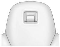
To fold a seatback forward, lift the latch on top of the backside of the seat. The seatback locks when folded down
