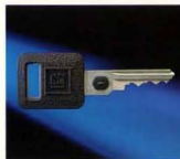
VATS EMPLOYS A DECODER AND IGNITION KEY WITH A PELLETT OF SPECIFIED RESISTANCE.
