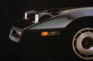
Powerful electric motors rotate the headlamps.
