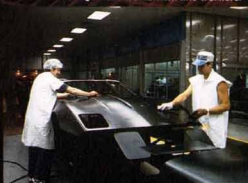
Meticulous wet and hand sanding are demanded by Corvette's tough paint inspection standards.
