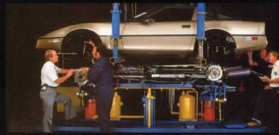
Specially built hydraulic towvee system "marries" chassis to body.
