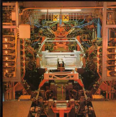
Two-stage welder builds uniframe.
