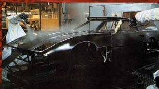
Robot painters apply base coat.
