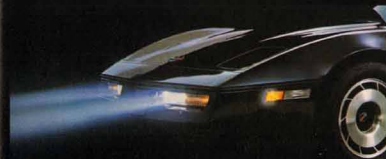
Integral halogen fog lamps operate independently of headlamps.
