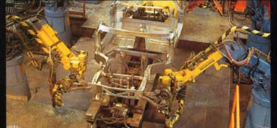
Uniframe components get additional precision robot welds.
