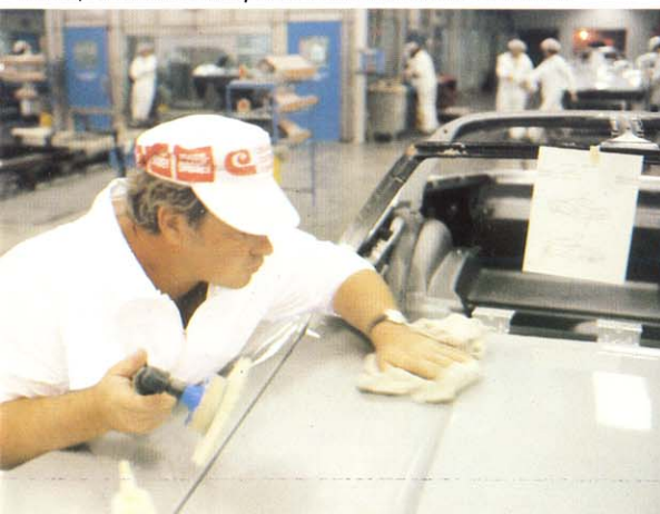
After a final clear coat, the finish is hand-polished and imperfections noted and removed.
