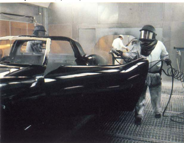
After a final clear coat, the finish is hand-polished and imperfections noted and removed.
