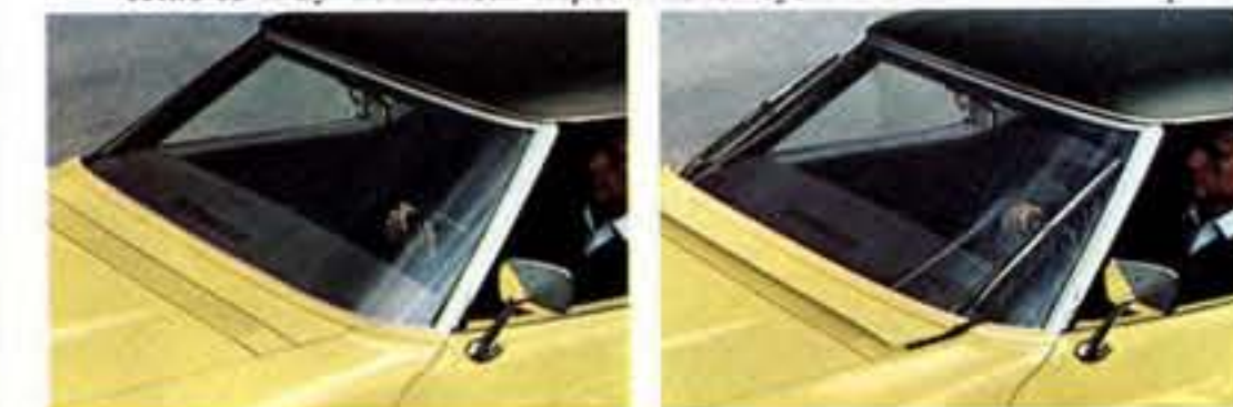
Hide-A-Way windshield wiper-washer system closed . . . and open.
