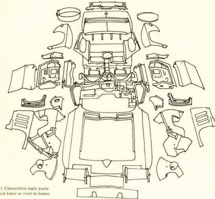
31 Convertible body parts that bond or rivet to frame
